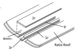
fashion the ridge on the roof ends but perhaps better, remove the whole ridge and then replace it with a strip of 0.5mm plastic across the whole arc. This can also help mask any visible join at the end. Roofs were painted white but became dark grey/black in service. A cast resin roof, S182, with the right length and profile is available from *Shire Scenes*
